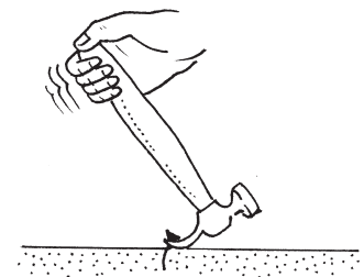
The hammer is acting as a force multiplier.
